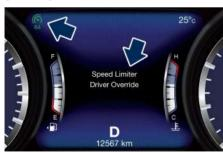
It is possible to do so at any driving speed, considering that it is possible to set a minimum speed of 30 km/h (18 mph).
