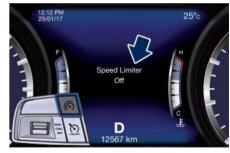
When the SL function is activated, the system automatically disengage the CC function if it was active.
