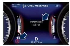
In this case, slow down until temperature returns to normal level (the light will turn off).
