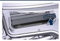
Close the filter access cover and reinstall the access door.
