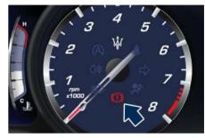
During engagement and disengagement procedures, the warning light (1) flashes until the parking brake has reached its maximum activation force and is respectively fully released.
