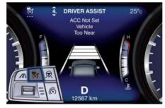
Push the ON/OFF button a second time and release to turn the system off. A pop-up message is displayed for
