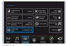
If TSA feature is set and a sign or a speed limit is detected, the related icons are displayed in the upper area of the instrument cluster beside of the main menu number and scroll arrows. The display area is divided in three different sectors:
