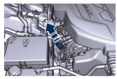
Re-insert the dipstick completely and remove: the oil level should maintain between the MIN and MAX reference ranges (SAFE range).
