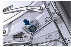
The brake pads wear could cause the fluid level to fall. However, low fluid
