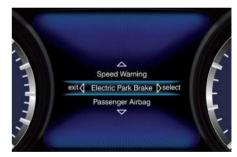
Press and release the switch once again toward the arrow ( ) to visualize the options connected to this function.
