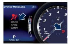
The air bag warning light monitors the internal circuits and interconnecting wiring associated with air bag system electrical components.
