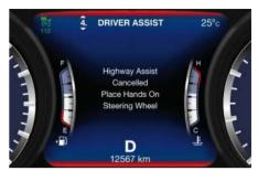
If the driver keeps his/her hands away from the steering wheel (for more than 8 to 10 seconds), also the ACC system is deactivated ( white ACC symbol on the display) and will have to be reset. The aid of LKA system will be disabled as well. In these cases the display will not show the attention level colour anymore and the vehicle will be controlled by the driver only.
