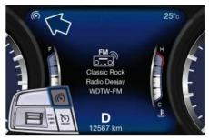
To disengage the system, push the same button a second time. The (S) light will turn off and a new message pops up for 5 seconds, then the display returns to the previous setting.
