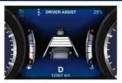
Remove foot from accelerator pedal and vehicle will continue at set speed.
