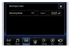
If the turn signal is then activated, and it corresponds to an alert present on that side of the vehicle, an audible chime will also be sounded: in the same moment the warning light will start flashing.
