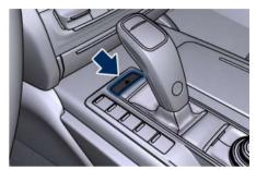
Press the switch to turn on the hazard warning flashers to warn oncoming traffic of an emergency. When these lights illuminate, the direction indicators, the related warning lights on the instrument cluster and the button start flashing.
