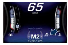
When the new gear is engaged, the indicator turns off. If the shift runs late or is not performed at all, the indicator remains lit for a few seconds then turns off. As soon as new conditions requiring further gear change occur, the indicator light will illuminate again.
