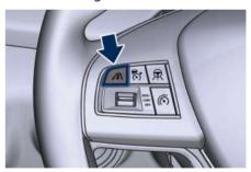
Each press and release of the button changes the gap starting from 3 bars (default distance) and moving in a sequential way towards the minimum distance:  $3\rightarrow2\rightarrow1\rightarrow4\rightarrow3\rightarrow2\rightarrow1\rightarrow4$  and so on.
