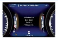
When the scheduled maintenance has overdue, the indicator light and message will be displayed on the instrument cluster.
