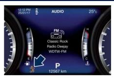
This warning light informs the driver that FCW is disabled. This warning light will light even when the activation of another driver assistance feature or drive mode (example: (ESC Off)) disables the FCW.
