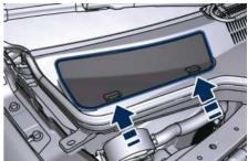
Unsnap both ends and lift the filter access cover.
