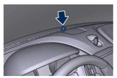
If the light remains on after the bulb check, it indicates that there is a problem with the electronics: this condition will result in the engine being shut off after two seconds. If the Vehicle Security Light turns on during normal vehicle operation (engine running for longer than 10 seconds), an electronic fault is detected. Should this occur, ask as soon as possible the **Service Network** for assistance.
