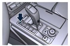
To deactivate the drive mode, press the same button again: the LED will turn off and the display will show the message indicating that  $\frac{1}{8}$  (ESC OFF) drive mode is off and ESC system is active.
