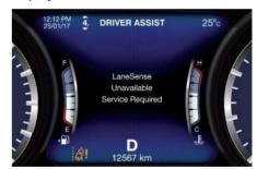
If message suggestion does not allow fixing the fault, avoid using the system and have the vehicle inspected at the **Service Network**.
