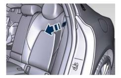
• Partially fold down the long seatback side and remove the head restraint of the center seat, by pressing at the same time the push buttons located at the foot of the head restraint. In this way it is avoided that the fully reclined seat back touches the edge of the central console.
