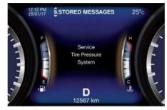
The instrument cluster will also display pressure values in place of the dashes (--). On the next ignition switch cycle the "Service Tire Pressure System" message will no longer be displayed as long as no system fault exists.
