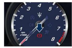
When parking on a hill, apply the parking brake before pressing the "P" button.
